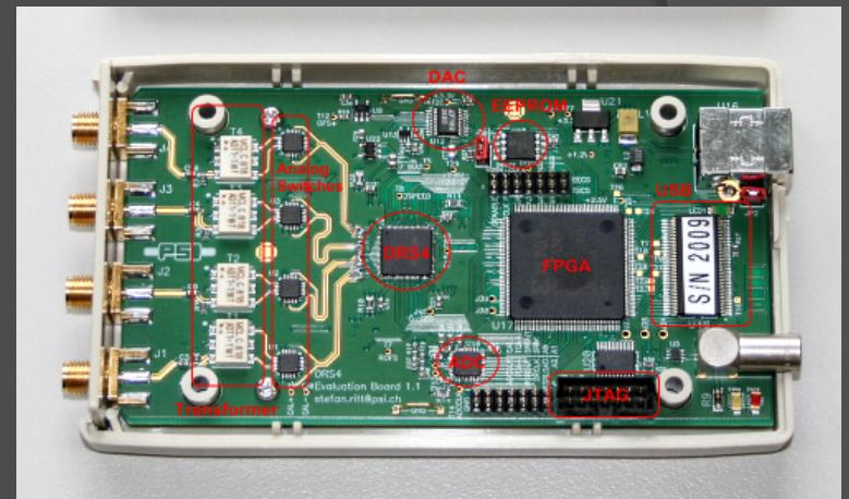
DRS4 can be operated from VME crate or stand alone with the DRS4 evaluation board
