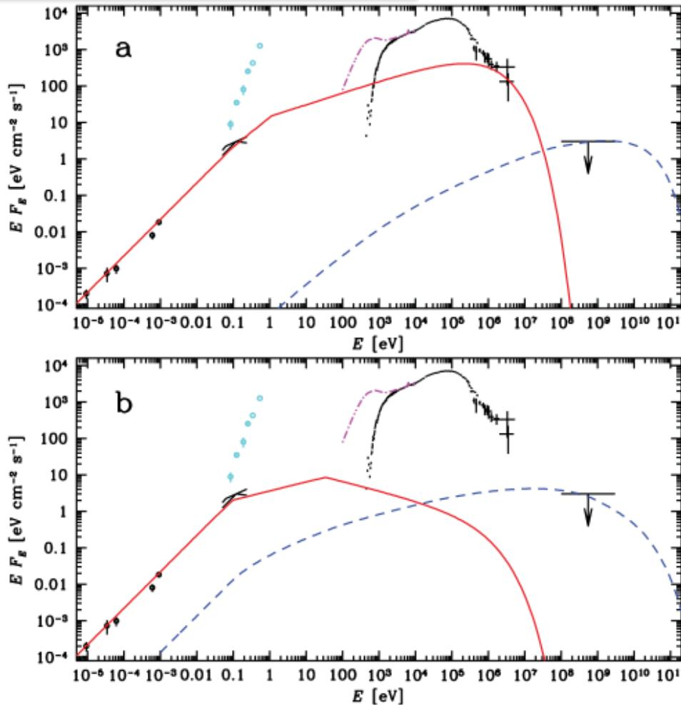
Figure 5. The data are the same as in Fig. 1. The red solid and blue dashed curves show the model synchrotron and Compton components, respectively. (a) Model 1 for  $p = 1.35$ , accounting for the observed MeV tail, which corresponds to the approximately maximum jet emission allowed by the data. (b) Model 2 for  $p = 2.5$ , in which case the jet emission is well below the MeV tail, which tail is then most likely emitted by hybrid plasma in the accretion flow. See
