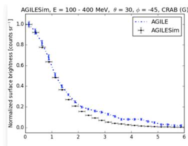
Figure 2. AGILE mass model (left panel) and comparison (right panel) between the simulated and detected PSF [6] in the 100 – 400 MeV energy range.
