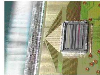
Silicon Tracker: 36864 Channels each with EN/DIS and threshold setting by TC or LUT at power On
