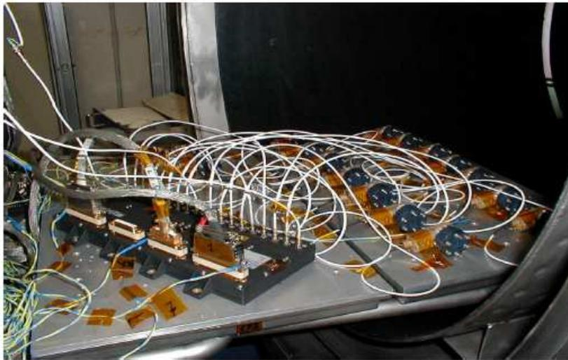
AC: 15 PMTs channels each ones with programmable HVs and gain
