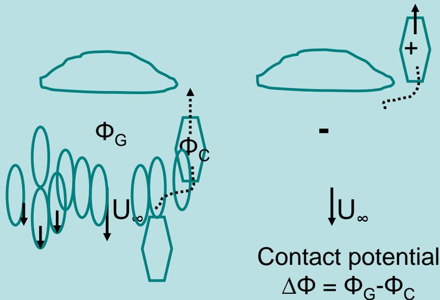
CHARGING DUE TO DIFFERENCES IN ELECTRIC SURFACE POTENTIAL BETWEEN THE TWO COLLIDING PARTICLES
