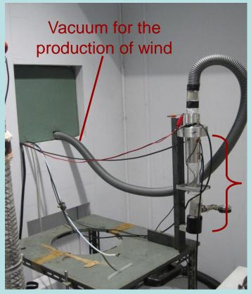
wind tunnel with three charge detectors
