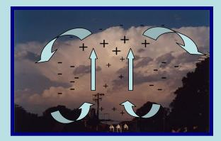
•DOWNDRAFT CARRIES NEGATIVE CHARGES TO THE EARTH SUFFICIENTLY TO INITIATE POSITIVE POINT DISCHARGE (CORONA EFFECT) WHICH ENHANCES THE POSITIVE CHARGE ENTERING THE CLOUD VIA UPDRAFT
