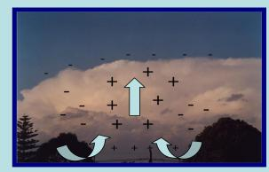
•NEGATIVE CHARGE SCREENING LAYER AT ITS TOP AND EDGES DUE TO CLOUD PARTICLE CAPTURE OF NEGATIVE IONS
