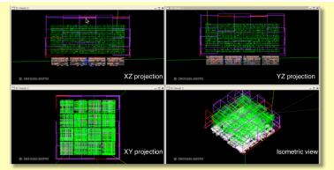
**Near peak of TGF**, LAT sees ~500 photons in ~5  $\mu$ s integration time, assuming typical RREA spectrum. Total energy deposited in calorimeter = 2030 MeV, distributed among ~500 photons.
