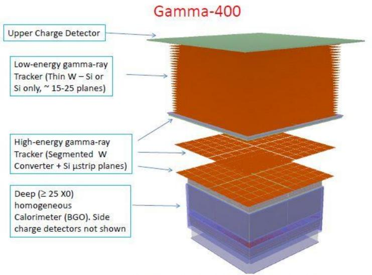
apparatus versions used in one of the preliminary simulations.
